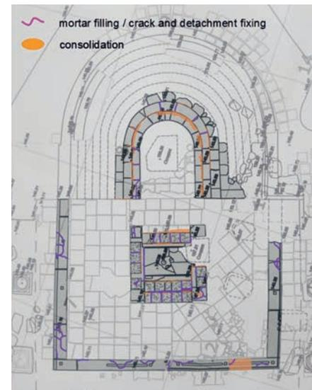
We started with mechanical cleaning of the area. Vegetation and dirt were removed, and we got a clear picture where to focus our future efforts. Due to the mechanical cleaning more cracks were revealed, and these were marked on the technical drawing. The next step was the consolidation of the material structure. Because of the annual changing of climate conditions, the lime mortar that holds the blocks was crumbling because the binder had lost
